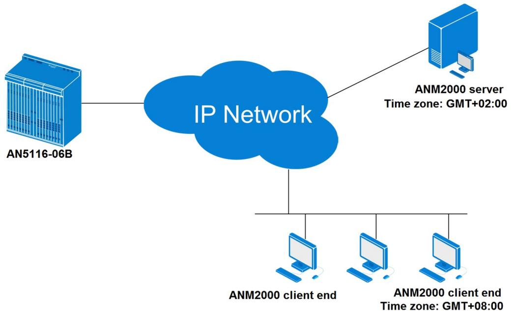
Figure 7-3 Network management server time asynchronous with the client end time in alarm report
