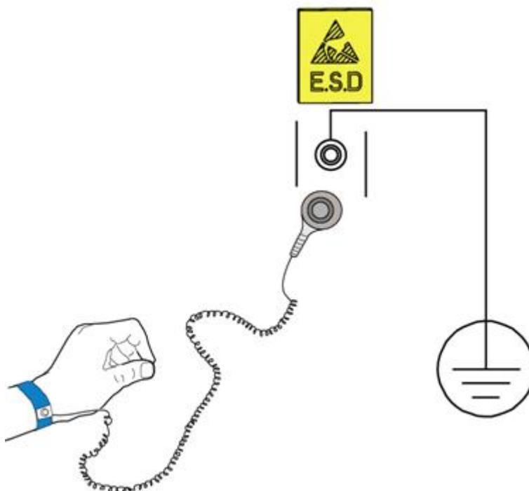
Figure 1-2 Wearing the ESD protection wrist strap
