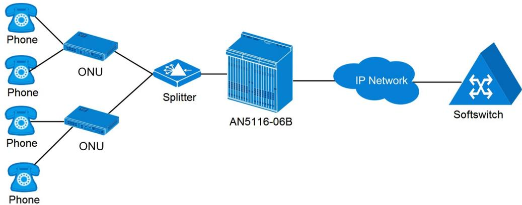
Figure 5-1 The AN5116-06B networking for voice service
