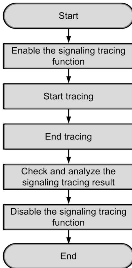
Figure A -1 Operation flow of signal tracing
