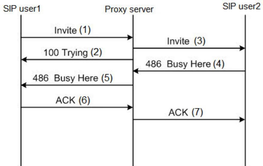
1. The SIP user1 initiates an Invite request to the proxy server. SIP user1 (77770001@132.108.95.1) of the proxy server (IP address being 132.108.95.1) calls SIP user2 (77770002@132.108.95.1). Below is the signal tracing example:
