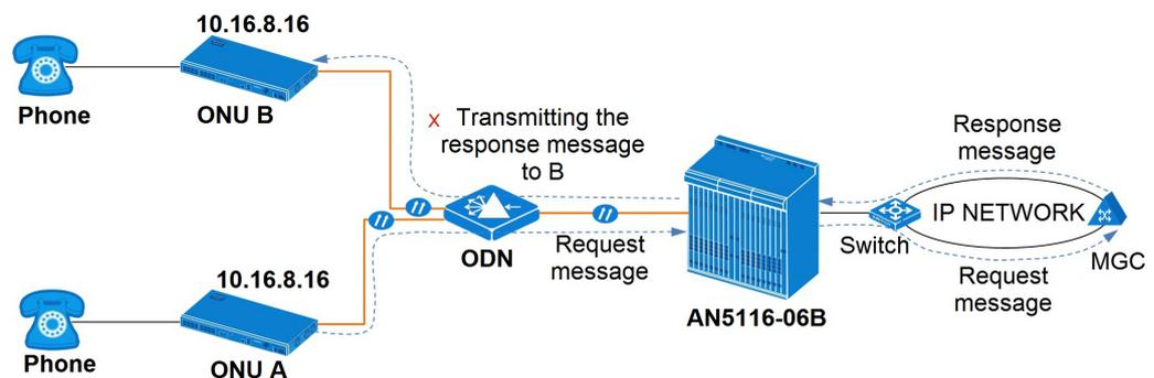
Figure 7-1 Frequent restart of endpoint
