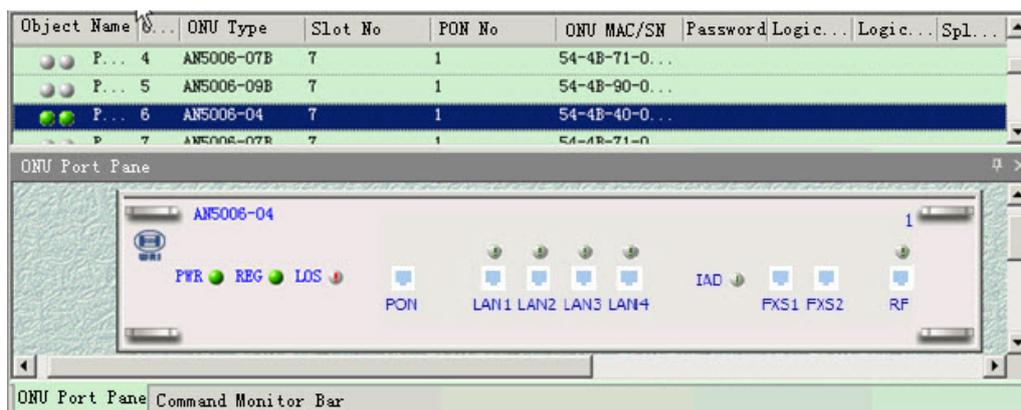
Figure 4-4 The GUI for checking ONU registration status
