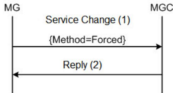
1. The MG sends the ServiceChange message to the MGC for logout. Below is the signal tracing example:
