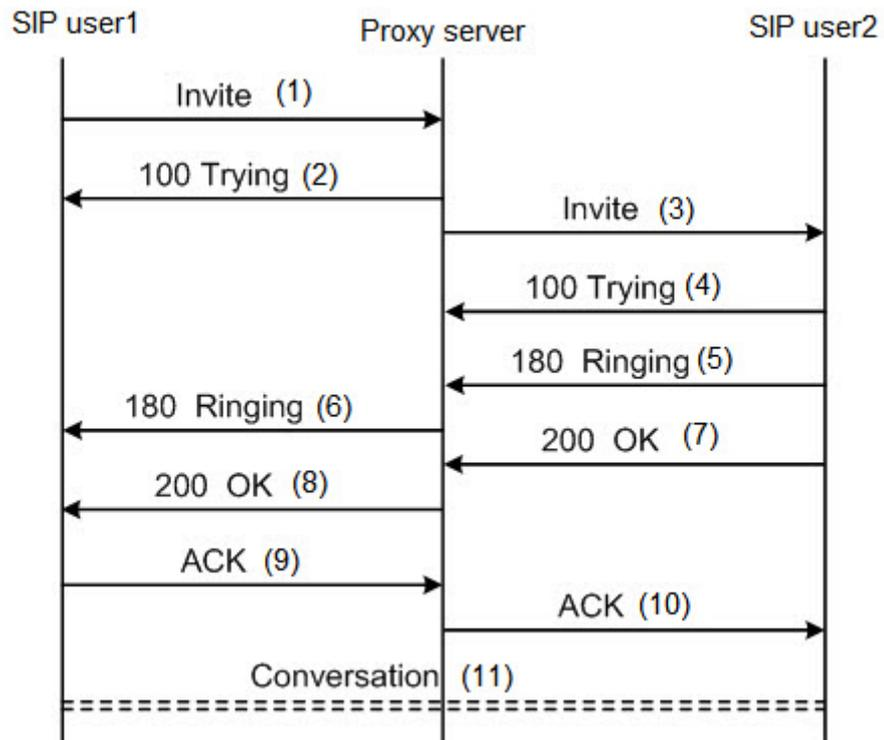
1. The SIP user1 initiates an Invite request to the proxy server. The “Allow” field of the request message lists the methods supported by the SIP user terminal, including Invite, ACK and Cancel; the “Content-Type” header field identifies the media type of the message body transmitted to the opposite party. Below is the signal tracing example:
