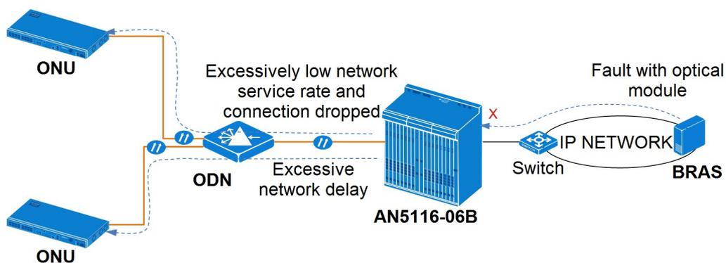
Figure 7-2 A majority of PON broadband subscribers under an OLT encountering faults in Internet service
