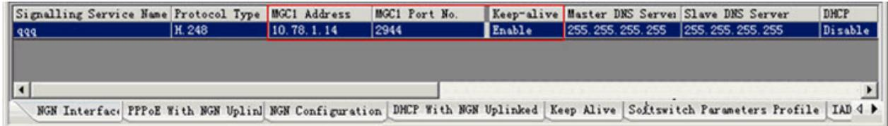
Figure 5-4 Checking the NGN uplink port configuration
