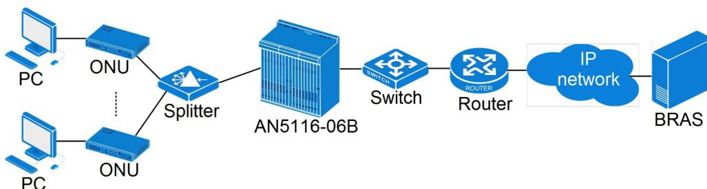
Figure 4-1 Typical networking of the AN5116-06B for data service
