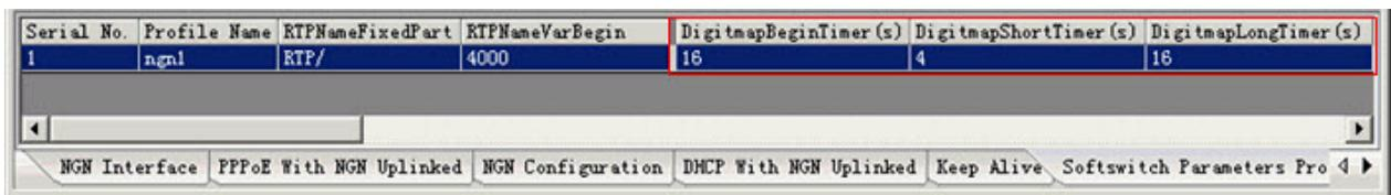
Figure 5-8 Checking the softswitch intercommunication template configuration (DigitMap timer)
