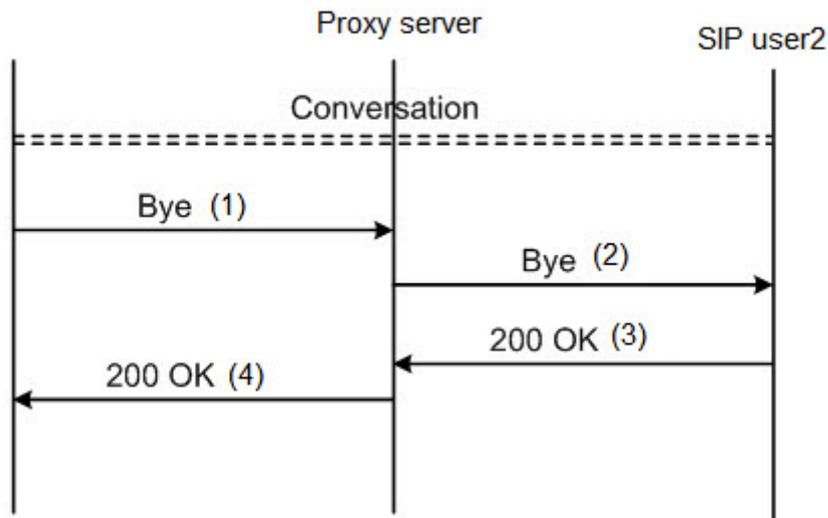
1. After the dialog is ended, the calling party SIP user1 hooks on and sends a Bye message to the proxy server. Below is the signal tracing example:
