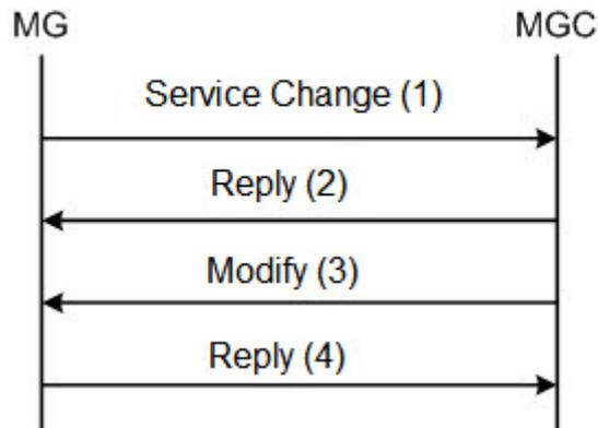
1. The MG sends the ServiceChange message to the MGC for registration. Below is the signal tracing example:
