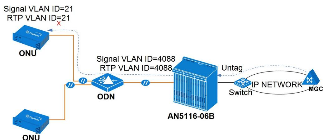
Figure 7-7 Subscribers under AN5006-20 ONU failing to hear the opposite party
