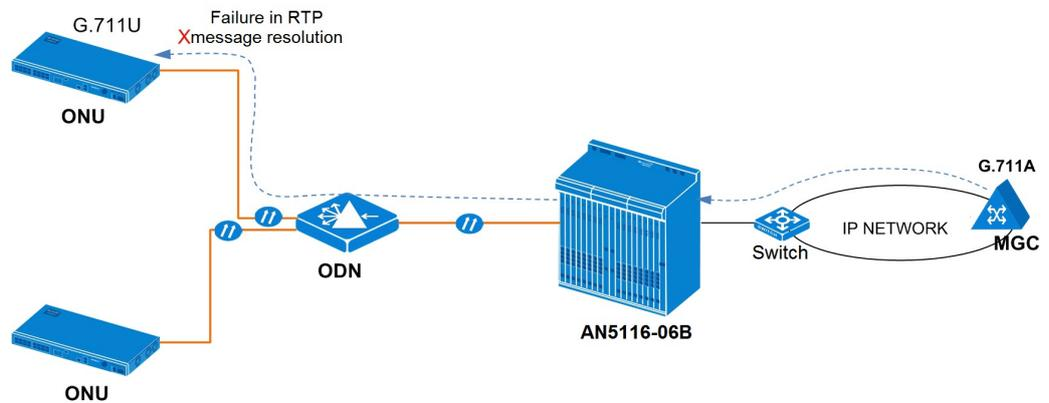
Figure 7-4 Voice encoding inconsistency causing abnormal connection of the subscriber as a called party
