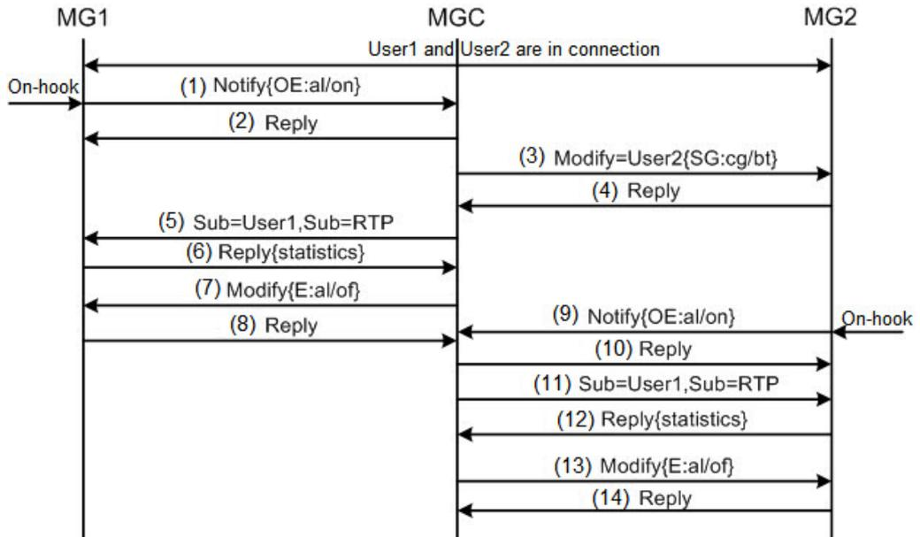
1. MG1 detects the off-hook of user a1 and reports the off-hook event to the MGC with a Notify message. Below is the signal tracing example:
