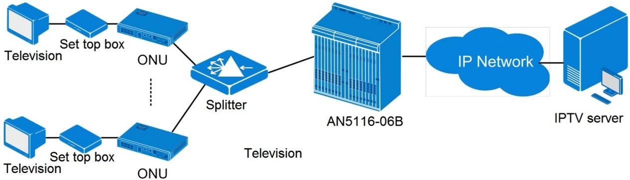
Figure 6-1 Multicast service networking
