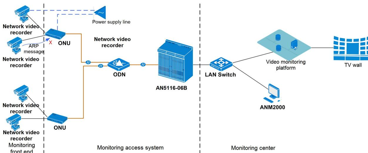
Figure 7-11 Video monitoring interrupted after power supply recovery
