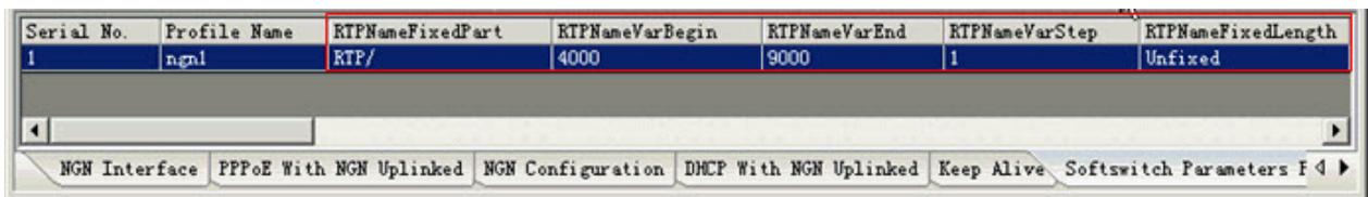
Figure 5-7 Checking the softswitch intercommunication template configuration (RTP resource)
