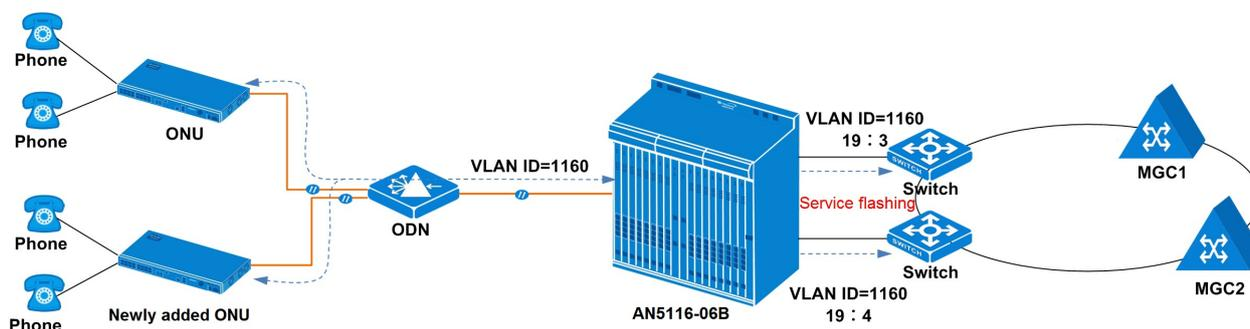
Figure 7-9 ONU reporting MGC disconnection alarm frequently
