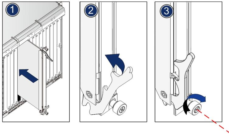
Figure 1-3 Installing a card
