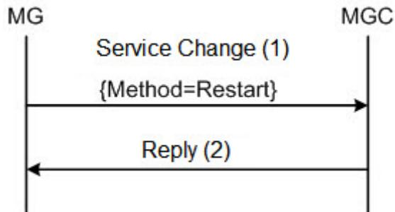
1. The MG sends the ServiceChange message to the MGC for registration. Below is the signal tracing information:
