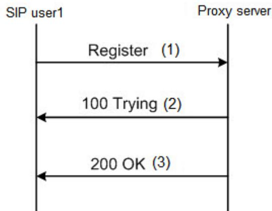
1. Before the first call attempt, SIP user1 should send the Register registration request to the proxy server. Below is the signal tracing example:
